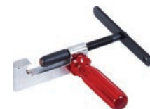
CT-204 Pinch-off Tool In extra strong execution to pinch-off suction tubes on all hermetic refrigeration systems up to 3/8" diameter.
